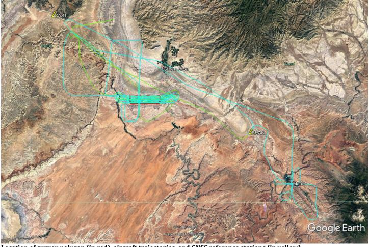
Location of survey polygon (in red), aircraft trajectories, and GNSS reference stations (in yellow)
