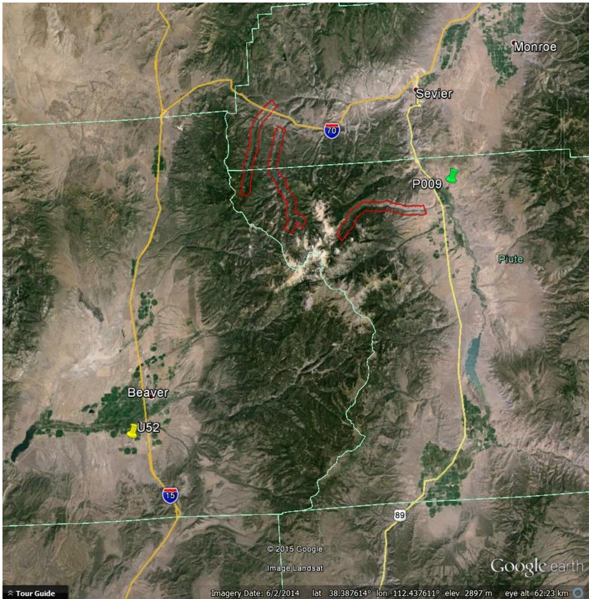
**Figure 1 – Location of survey passes over the streams (corridor polygons in red). P009 and U52 show the location of GPS reference stations. (Google Earth).**
