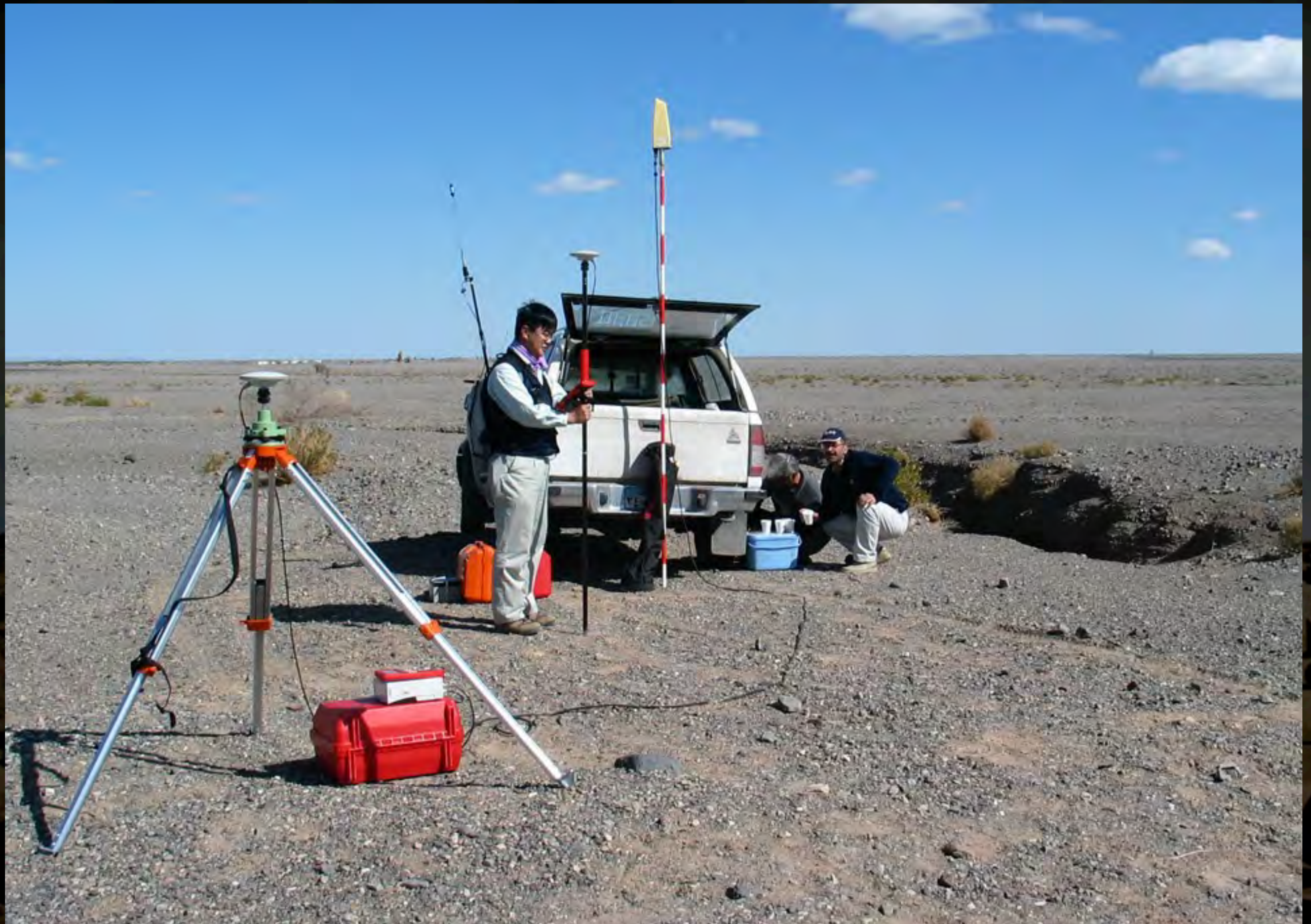
RTK-GPS radio modem setup (Bam, Iran, 2004)
