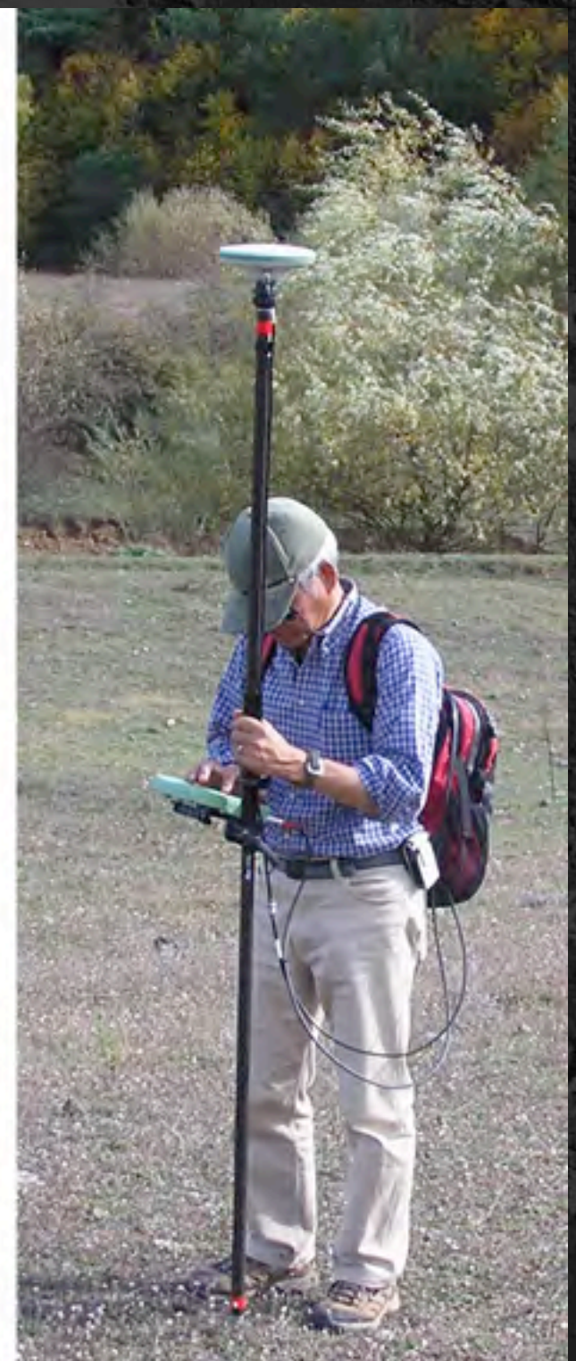
Rover: static stop and go 5 sec.
