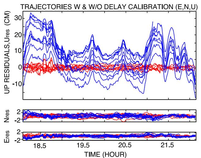
**Figure 3.** The up, north, and east residual time series associated with the eleven initial solutions derived using the default delay model (blue curves) and those associated with the refined solutions derived using the externally calibrated delay model (red curves). The residuals are defined relative to the mean of the refined solutions.
