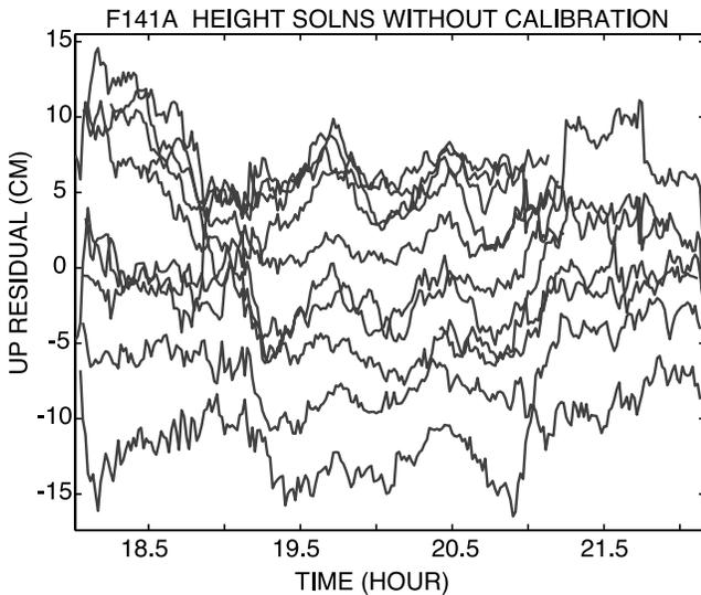
**Figure 1.** The height residual time series associated with each of the aircraft trajectory solutions obtained using 11 different base stations. The average of the eleven trajectory solutions was removed from each single base station solution to form the residual time series for that base station.
