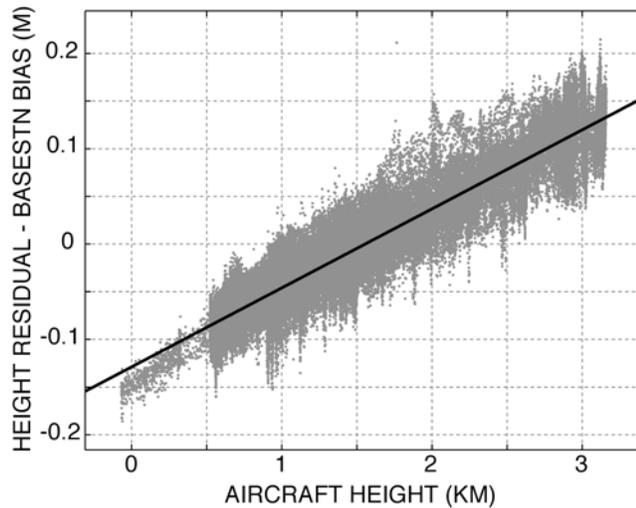
**Figure 4.** The non-steady component of height error in the original height solutions, defined as the residual height time series (blue curves in Figure 3) minus the mean value of that series for each base station, plotted against the instantaneous height of the aircraft. The data for all 11 solutions are plotted together. The best fitting straight line has a gradient of  $8.29 \pm 0.01$  cm/km.
