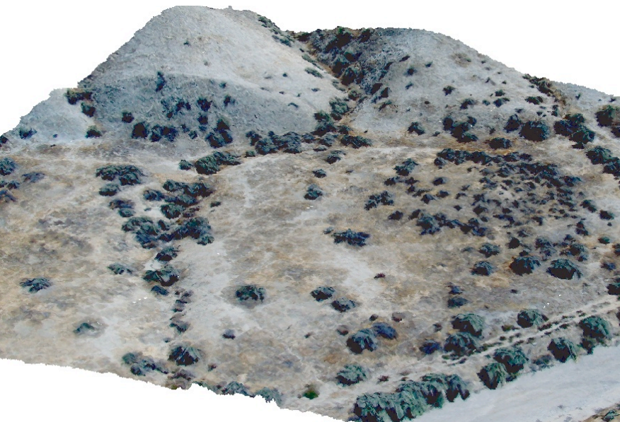
LiDAR/imagery fusion: 4 cm pixel balloon aerial photo merged with 25 cm B4 DEM.
