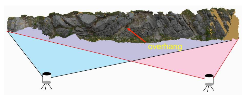
Choose scan positions to minimize occluded (shadowed or hidden) geometries.
