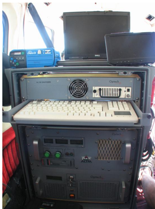
Figure 1 – NCALM Gemini ALTM and digitizer installed in the Cessna Skymaster N337P.
