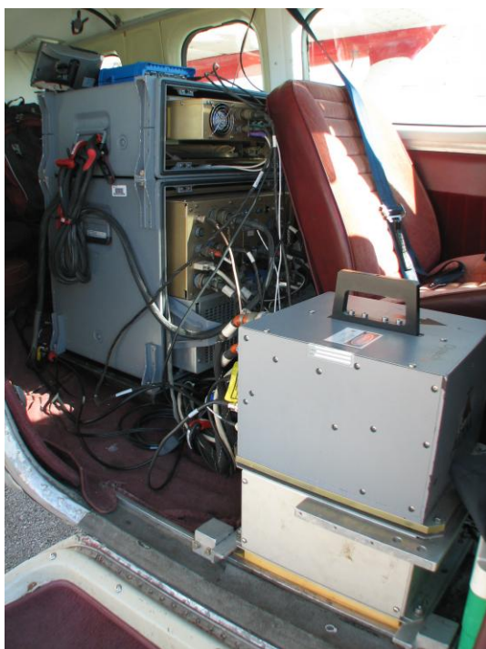
Figure 1 – NCALM Gemini ALTM and digitizer installed in the Cessna Skymaster N337P.
