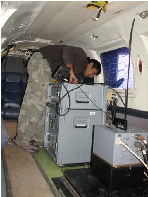
Figure 1 – NCALM Gemini ALTM installed in a Piper PA-31.
