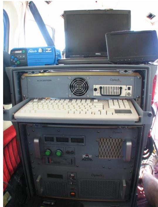
**Figure 1 – NCALM Gemini ALTM installed in the Cessna Skymaster N337P.**
