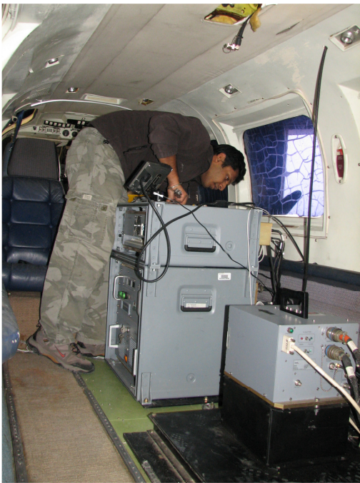
Figure 1 – NCALM Gemini ALTM and waveform digitizer installed in a Piper PA-31.
