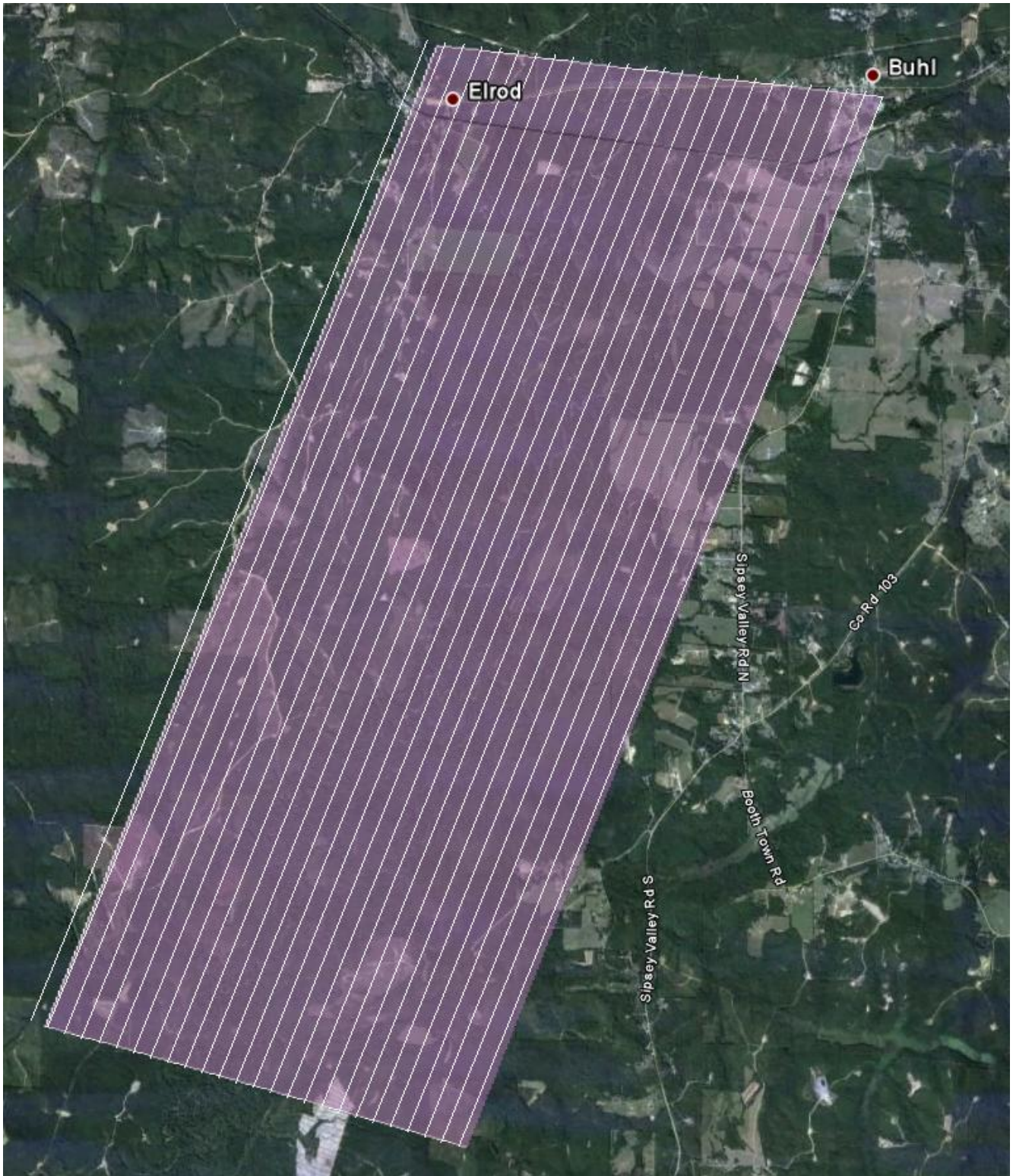
Figure 3 – Extent of survey polygon with flight lines (Google Earth).
