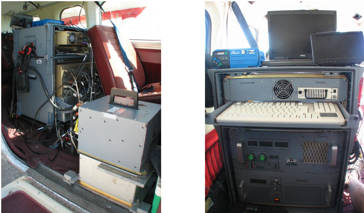
Figure 1 – NCALM Gemini ALTM and digitizer installed in the Cessna Skymaster N337P.
