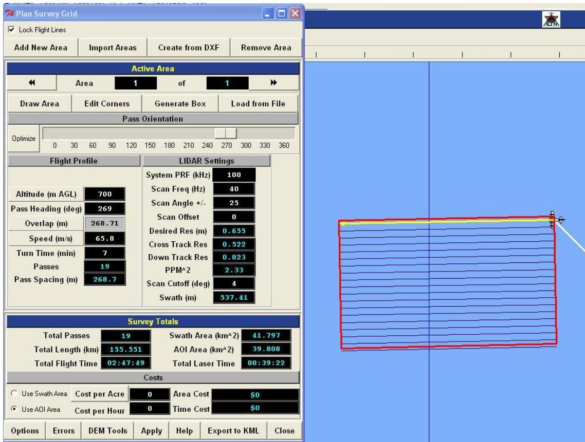
Figure 2 - Flight lines with planning parameters.
