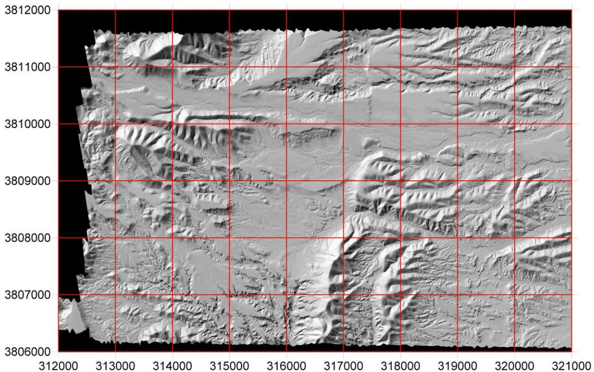
**Figure 4 - Tile footprints overlaid on a shaded relief image of the bare-earth DEM.**
