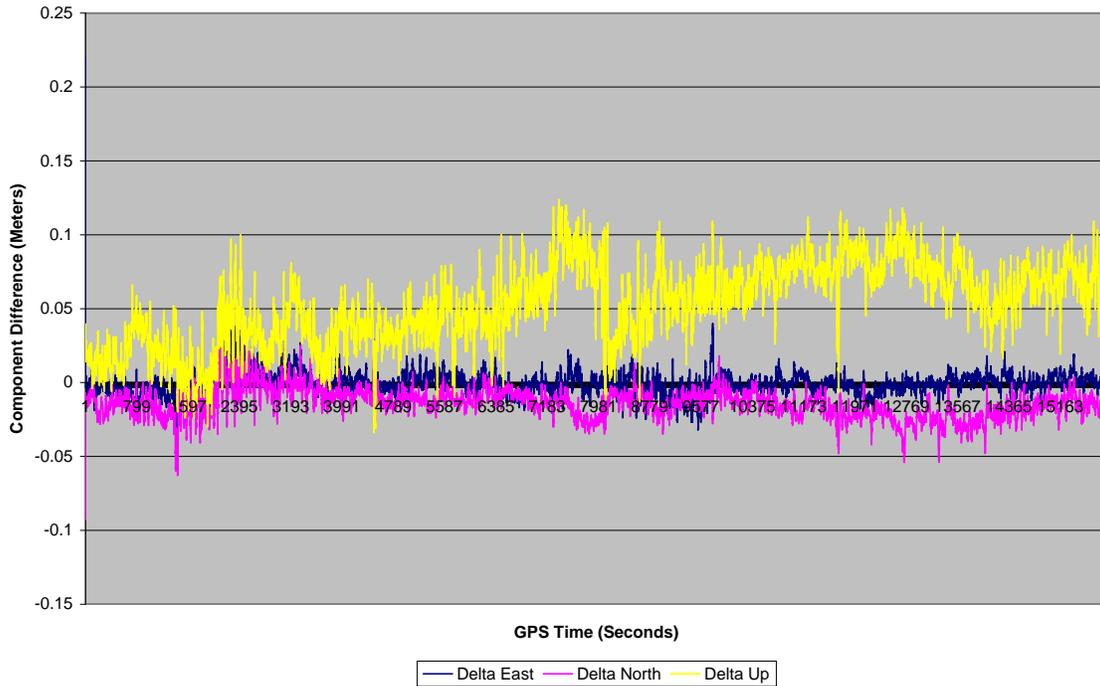
Figure 3 - Positional differences in aircraft trajectories with respect to time as processed from 2 base stations.
