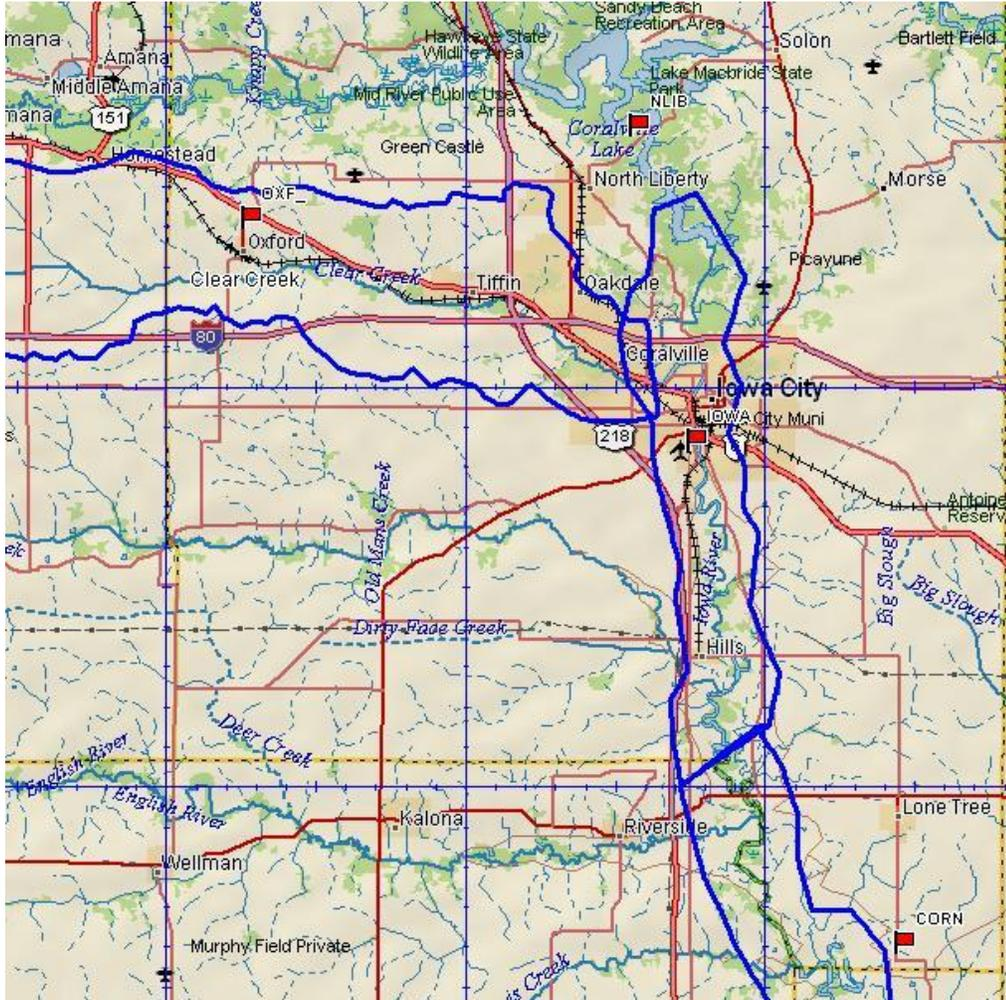
Figure 5 - Red Flags show locations of GPS reference stations used for trajectory processing.
