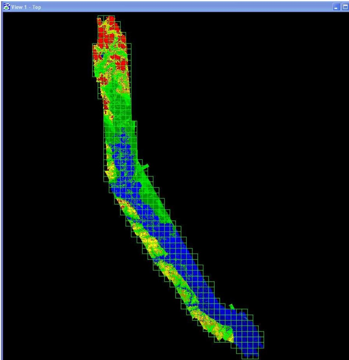
**Figure 7 - Tile footprints overlaid on the point cloud colored by elevation.**
