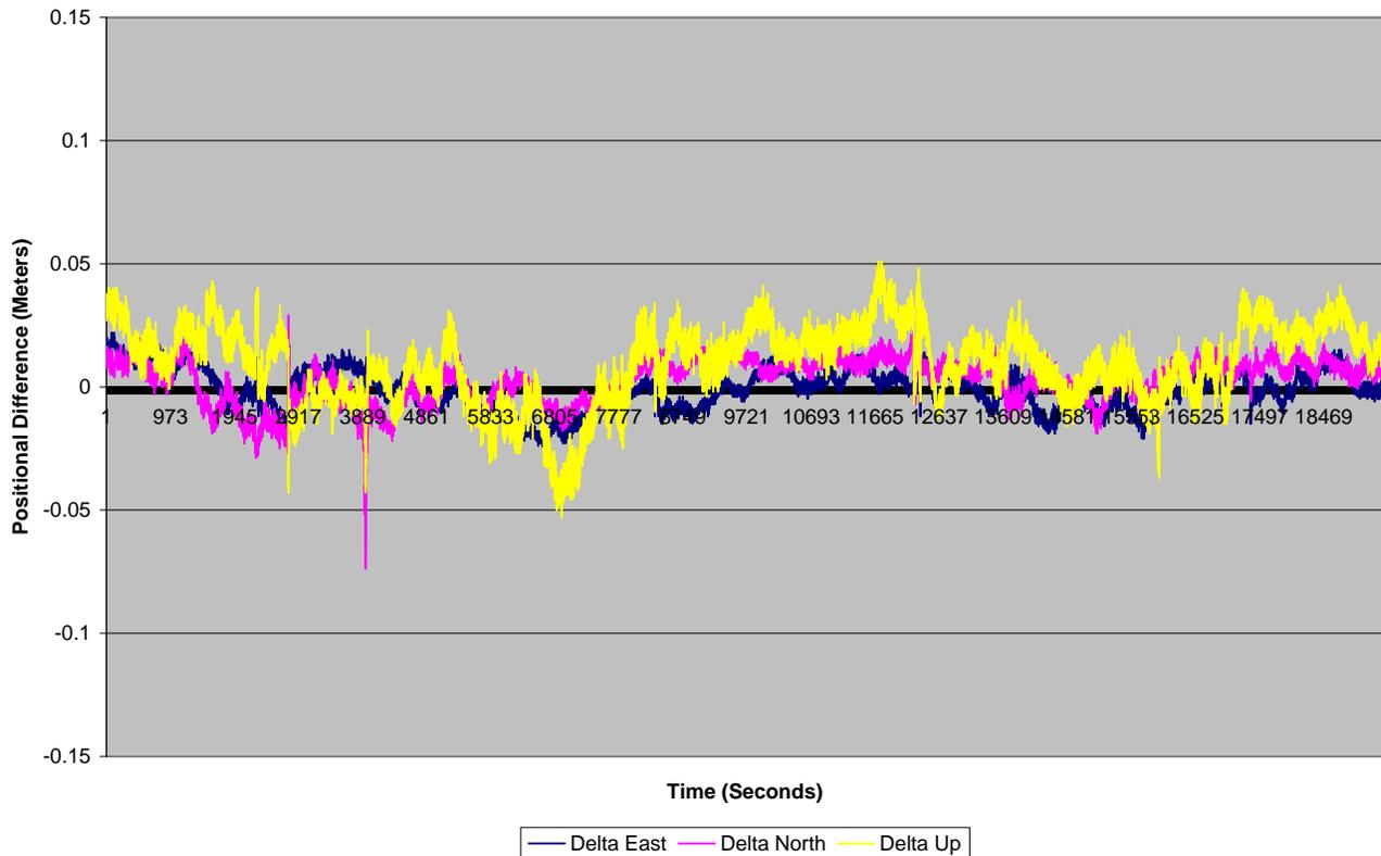
**Figure 6 - Positional differences in aircraft trajectories with respect to time as processed from IOWA and CORN**
