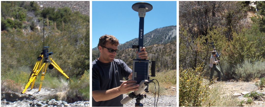
Figure 2. RTK surveys utilize a base GPS unit that is set up and connected to a radio and antenna. The roving GPS unit is attached to a field data logger and receives a kinematic correction to collect field RTK data.
