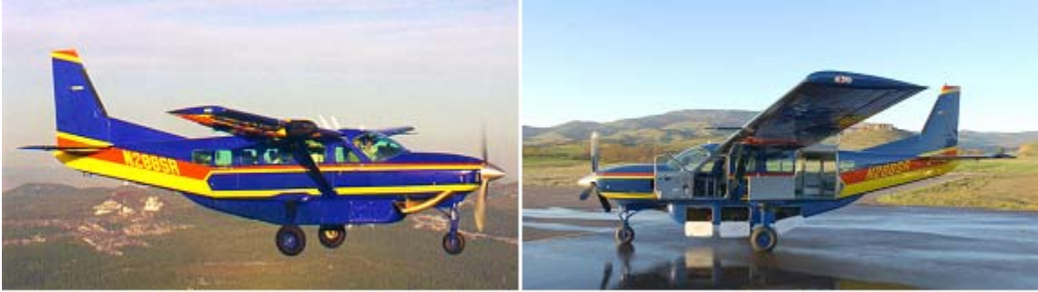
Figure 2. The Cessna Caravan 208 - A removable composite cargo pod provides housing for GPS equipment and the LiDAR system and other remote sensing equipment.
