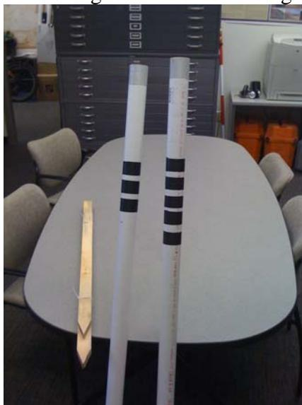
**Figure 2.** Two examples of the targets and stakes used to help align the TLS scans.
