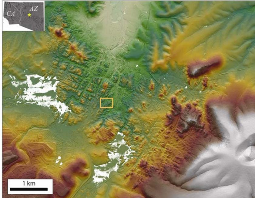
**Figure 1.** Location map of the TLS survey area. ALS-generated 0.25 m DEM of the Granite Dells precarious rock zone was collected by the National Center for Airborne Laser Mapping (NCALM; <http://ncalm.org>) for a Seed Grant. Modified from Haddad (2010).
