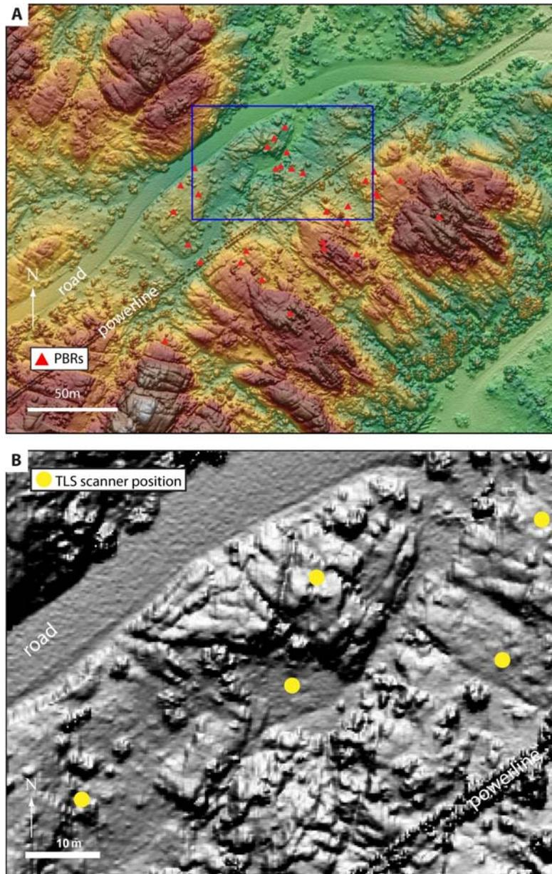
**Figure 3.** Location map of TLS scanner positions used to scan a small channel and adjacent hillslopes. (A) Overview hillshade created from an airborne laser scanning (ALS)-generated 0.25 m digital elevation model (DEM). Blue box outlines the TLS survey area. (B) Location map of the TLS scanner setups. A total of five scan setups were used to scan the ~60 m by ~100 m area covering PBRs, surrounding hillslopes, and a small channel. Modified from Haddad (2010).
