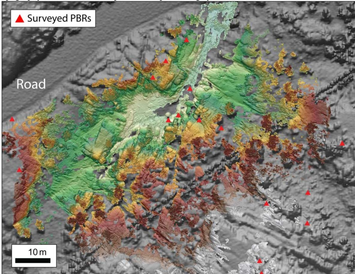
**Figure 4.** A 0.05 m DEM of the TLS survey area nested in a 0.25 m ALS-generated DEM. Modified from Haddad (2010).
