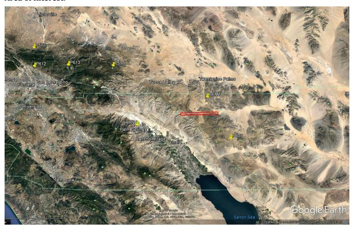
Location of survey polygon (in red) and GNSS reference stations (yellow push pin markers)
