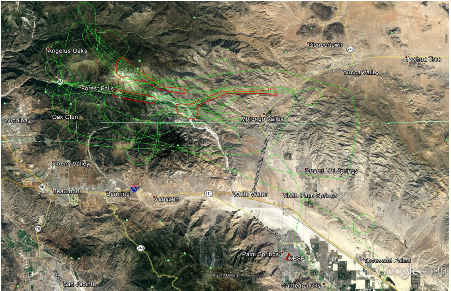
Location of survey polygons (in red), aircraft trajectory (in green), and GNSS reference station
