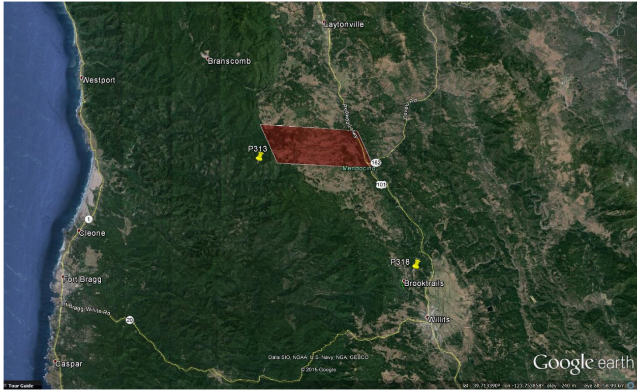
Figure 1 – Location of survey polygon (in red). Yellow push pins represents the locations of GPS reference stations P313 and P318. (Google Earth).
