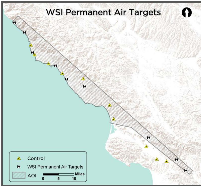
Map of permanent air targets painted by WSI in the San Simeon project area. In addition to permanent air targets painted by WSI, other permanent targets were identified in the field and used for rectification of orthophotos during processing.
