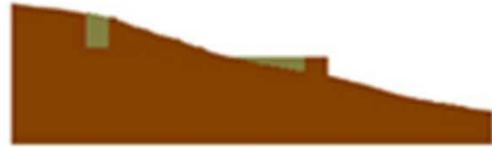
Pit Removal (Filling)
